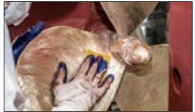
Sanding metallic surface with 80 grit sandpaper.
