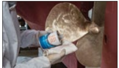
Clean surface with acetone.
