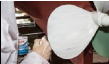
Applying first coat of Velox Plus paint.
