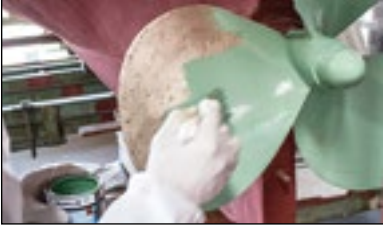
Applying Metal Primer.
