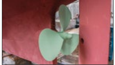
After applying Metal Primer.
