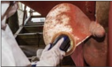
Removing old antifouling.
